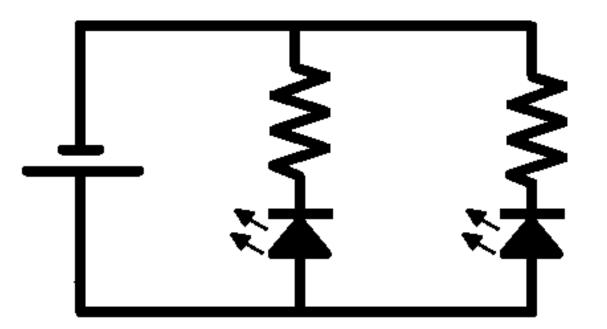
In this circuit you will have two LEDs, and one resistor apiece, the objective is to make them work together at the same time
