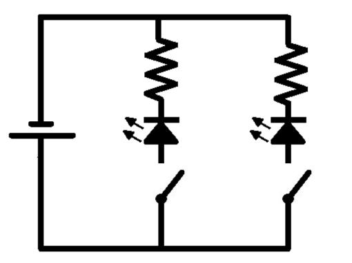
In this exercise you will have to assemble two LEDs, two resistors to keep the current through the LEDs under control and two buttons, each of them will manage one of the LEDs
