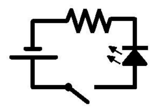
This exercise adds a button, so the LED will switch on only when the switch is being pushed
