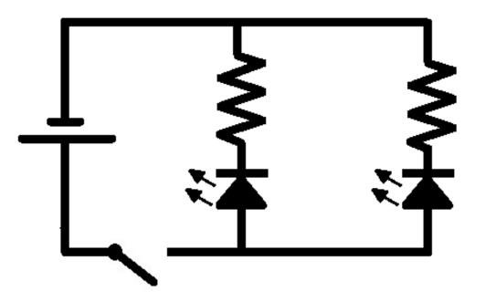
This exercise has a button that has an effect on both LEDs in the circuit, the switch will turn both LEDs on (if pushed) or off (if released)
