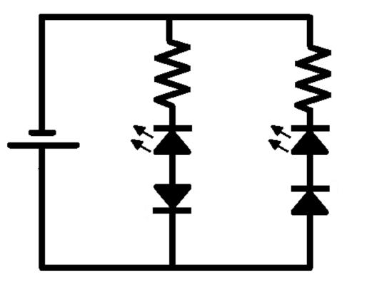
In this exercise you will assemble two LEDs and their resistors and a diode along with them but the diodes must be in opposite positions. This will prevent one of them to turn on.
