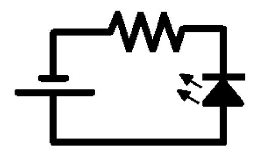
In this exercise you will have to turn on the LED, which will be assembled along with a resistor
